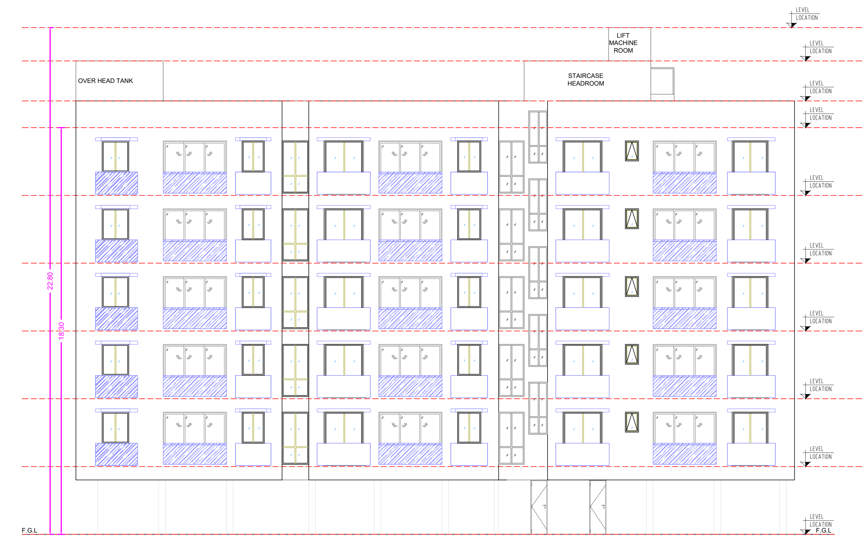
SOUTH SIDE ELEVATION BLOCK - A
