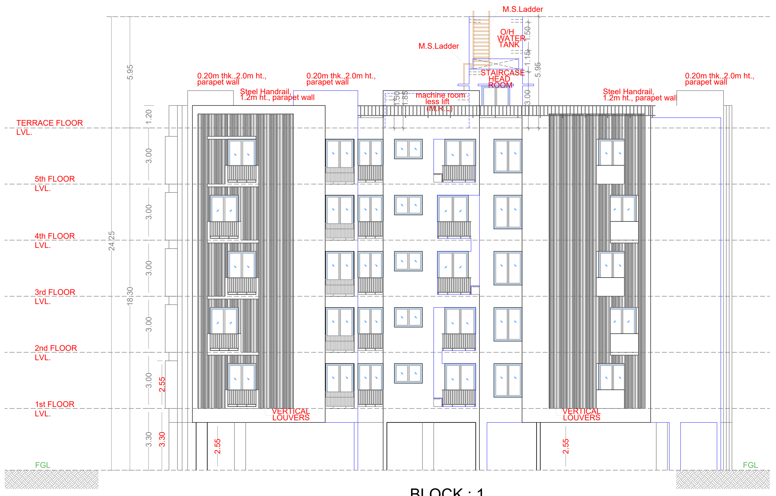
BLOCK : 1 WEST SIDE ELEVATION
