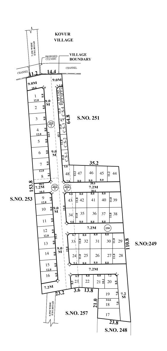
SITE EXTENT (AS PER PATTA) 7550 SQ.M **ROAD AREA** 2829 SQ.M PUBLIC PURPOSE PROVIDED (1%) PP-1 HANDED OVER TO THE LOCAL BODY (0.5%) = 26.0 SQ.M PP-2 HANDED OVER TO THE TANGEDCO (0.5%) = 25.0 SQ.M TOTAL NO. OF PLOTS **CONVENIENCE SHOP SITE** 4 Nos **NOTE:** 1. SPLAY - 1.5M x 1.5M 2. MEASUREMENTS ARE INDICATED EXCLUDING SPLAY DIMENSIONS 3. ROAD AREA
